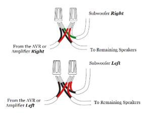
We recommend that you use only multi-strand direct burial wire. The gauge of the wire will depend on the length of the run. Check our website for wire gauge recommendations.
