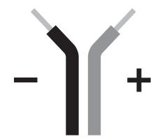
It is very important that the same wire that is attached to the Positive connector of the Audio Source is attached to the Positive connector of the speakers.
